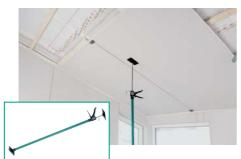
The integrated moving hook on the lifter makes it easier to assemble the boards on the wall.
