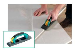
Resulting cut or broken edges are subsequently smoothened with the edge planer. Straight cut edges are chamfered to around 2/3 of their density before the boards are fixed. Edges that have already been chamfered can be easily broken using abrasive paper.
