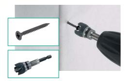
The plasterboards are fastened to the wooden strip, squared timbers or a metal post-and-beam structure using special dry wall screws. These are available with a fine thread for frame sections and stud profiles and a coarse thread with different lengths, depending on the thickness of the plasterboards, for wooden ledges or squared timber. A cordless screwdriver with electronic speed control and a screw attachment with depth stop is the ideal tool for this job.
